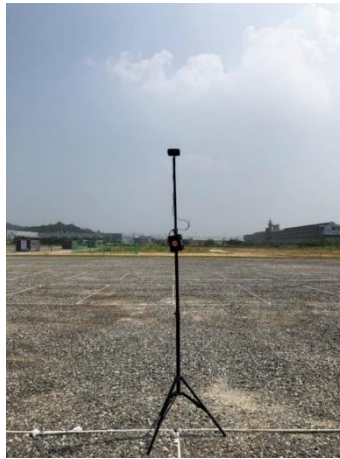
Figure # 13 RTK Base Installation
